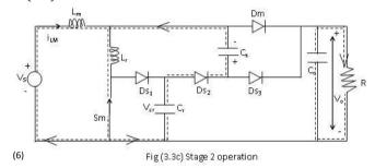
From the circuit of second stage of operation, three equations can be derived with regard to resonant capacitor voltage, resonant inductor current and snubber capacitor voltage as follows;
