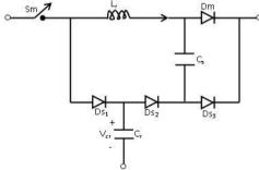
Fig (3.1) passively soft switching dircuit cell
