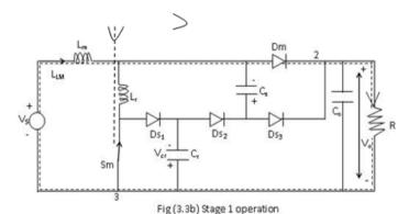
$$-V_{32} = \frac{L_r di_{Lr}}{dt} = V_0^{(5)}$$
