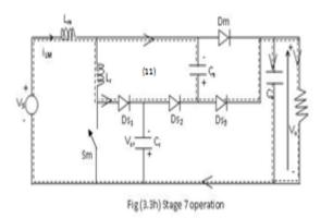
Thus the resonant inductor current is further decreased until it becomes zero at t<sub>2</sub>, thus causing the whole of I<sub>2</sub> to flow through C<sub>s</sub>. That is,
